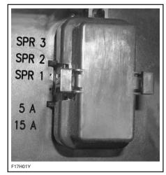
FUSE IDENTIFICATION 5 A: MPEM 15 A: Battery
